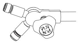
Flexible balljoint adjusts your device to desired positions by loosening/tightening the adjustment knob.
