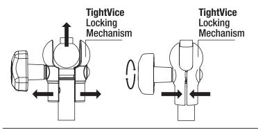
How TightVice™ & 360° Locking Mechanism works: Use the adjustment knob to position the ball joint at the desired angle. Tighten to make sure your microphone or device is held in place.
